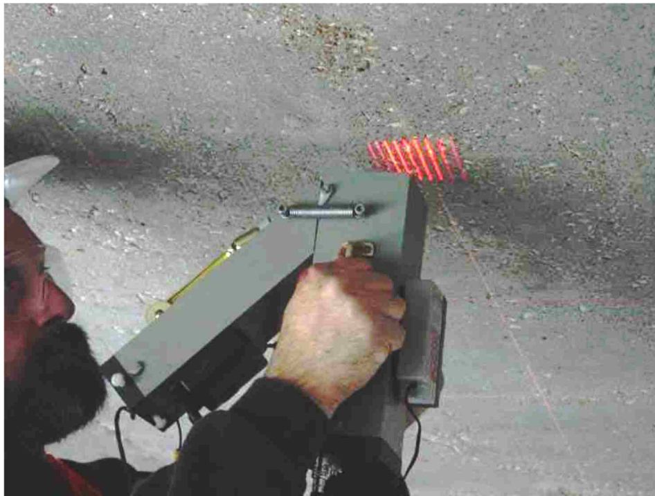
Figure 2.7. Laser Profilometer (Holdener et al. 2004)
