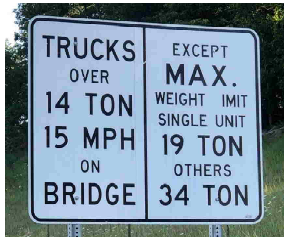
Figure 3.1. Bridge P-0058 Load Posting
