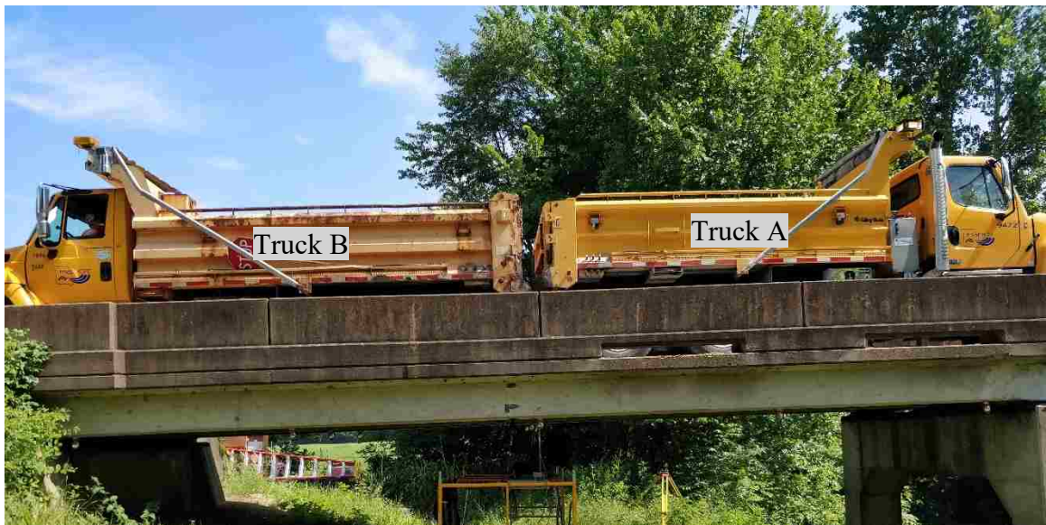
Figure 5.7. Trucks on Span 1 for Load Test
